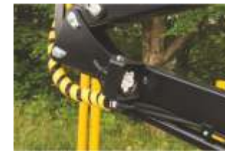
LED lights on crane
